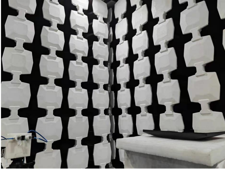
Description: Radiated Emission Test Setup (Above 18GHz)
