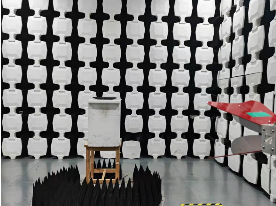
Description: Radiated Emission Test Setup (1GHz -18GHz)
