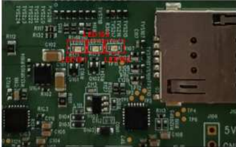
Feature 12: LED status indicator light (LED101、LED102、LED103)
