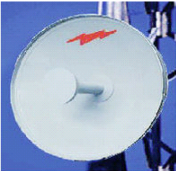
PX4F-52-NXA/A 1.2 m | 4 ft Standard Parabolic Unshielded, Dual-Polarized Antenna, unpressurized, 5.250–5.850 GHz, N Female, gray antenna, molded gray radome with flash, standard pack—one-piece reflector
