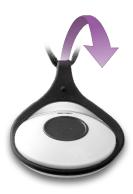
2. Twist a coin in the slot to open the cover.
