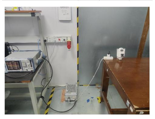
Conducted emissions at AC power line (150kHz-30MHz)
