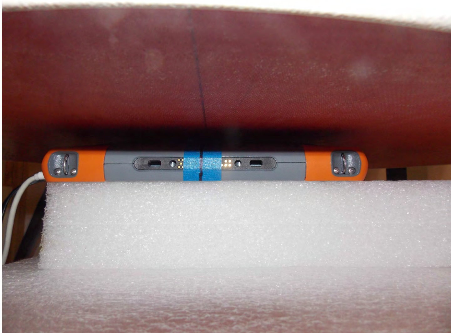
Test Position RFID Back 0 mm Gap
