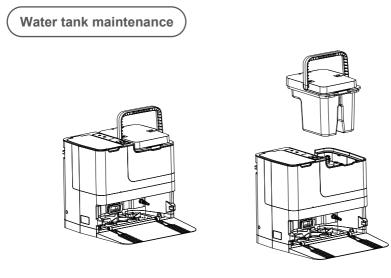
Pull up the handle of the water tank, lift the water tank vertically and take it out.
