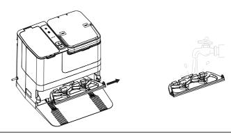
Pull up the mop cleaning bracket, clean it with water and put it back into the base station.
