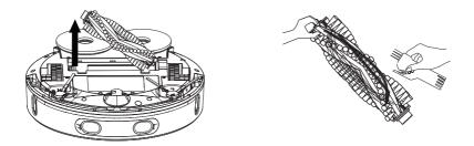
Take out the roller brush shaft and clean the impurities and hair on the roller brush shaft.
