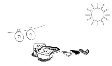
Dry the dust box and filter components and keep them dry to ensure their service life. When the lifting tank is used for 15-30 days, it is recommended to wash it once. The maximum service life of high efficiency filter is 3 months.
