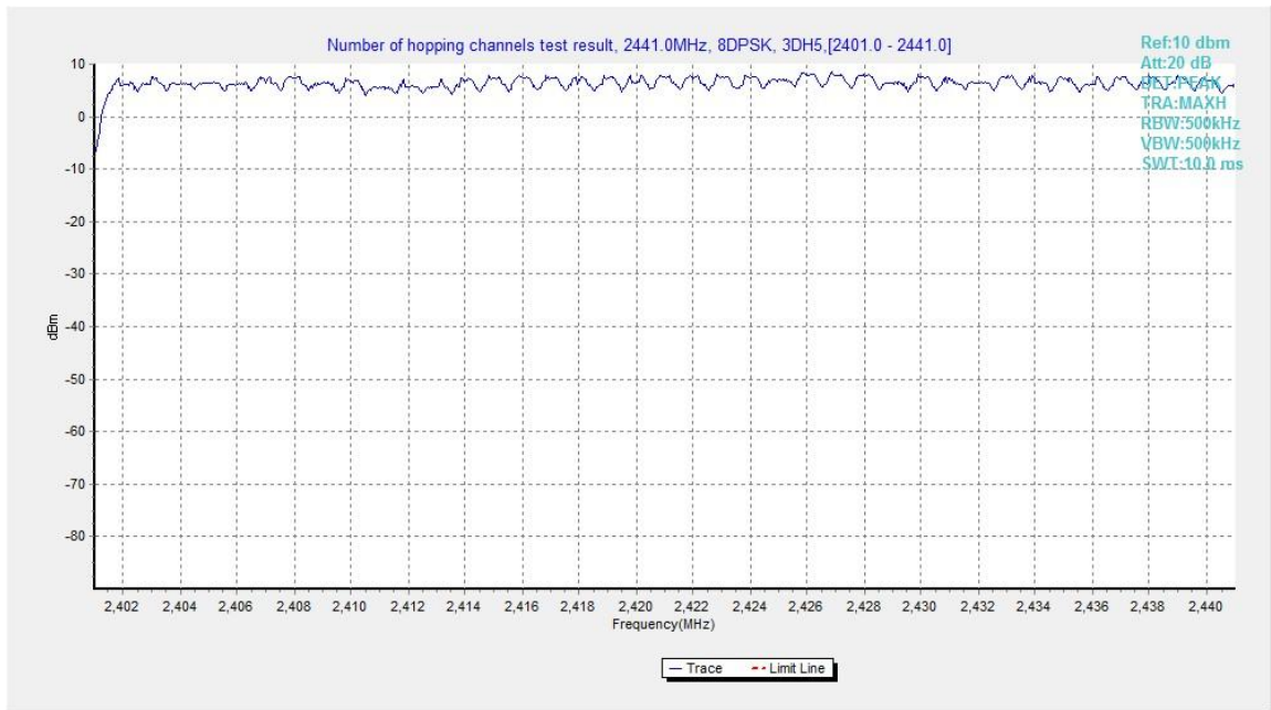
Fig.98. Number of hopping frequencies: 8DPSK, Channel 0 - 39
