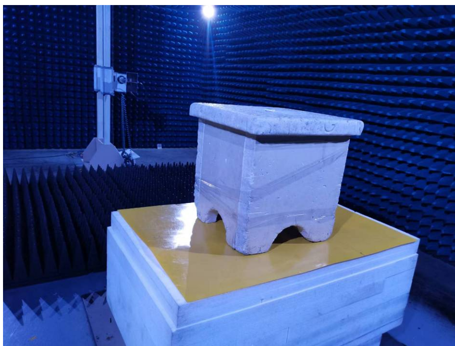
Photo of Radiated Emission Measurement (Above 1G)
