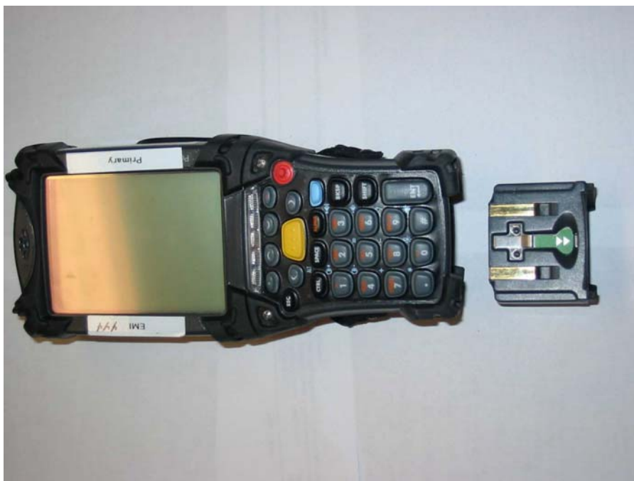
Figure 4 – MC9063 with Battery Removed
