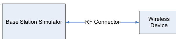
Figure 9-1 Power Measurement Setup
