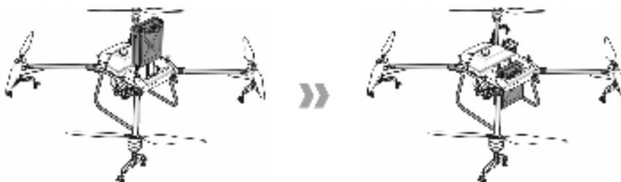
Figure 1-11 Install the battery
