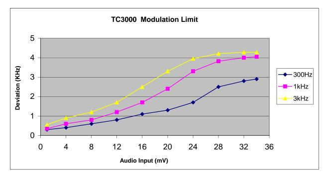
For 12.5KHz Channel Spacing:
