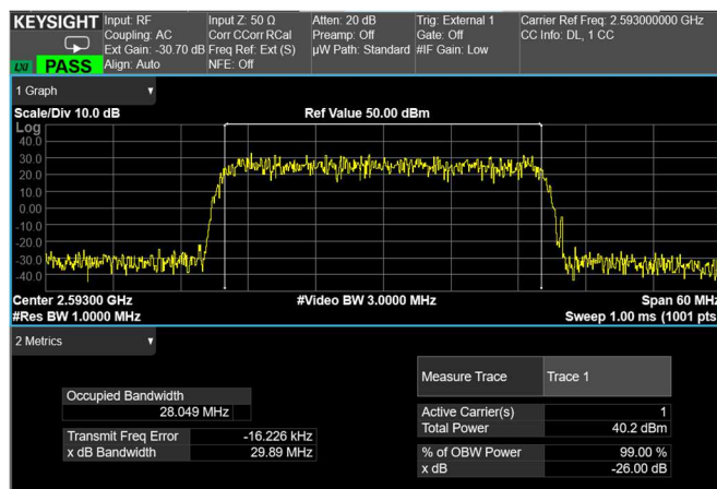
Channel: MIDDLE, Modulation: 64QAM, BW=30MHz
