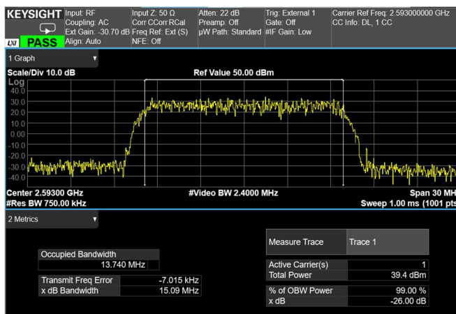
Channel: MIDDLE, Modulation: 64QAM, BW=15MHz
