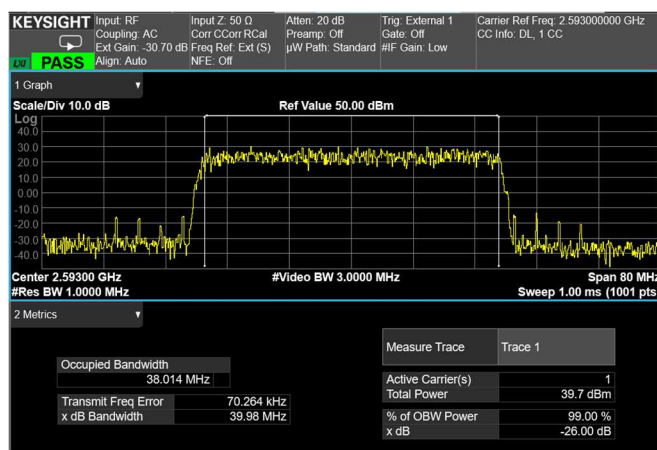
Channel: MIDDLE, Modulation: 64QAM, BW=40MHz
