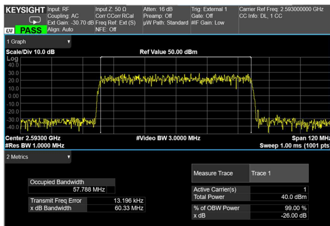
Channel: MIDDLE, Modulation: 64QAM, BW=60MHz
