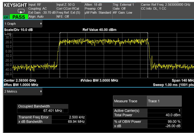
Channel: MIDDLE, Modulation: 64QAM, BW=70MHz
