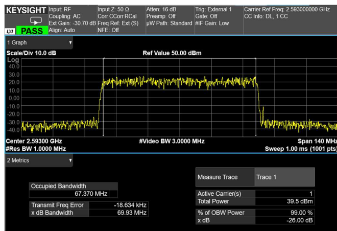
Channel: MIDDLE, Modulation: 64QAM, BW=70MHz
