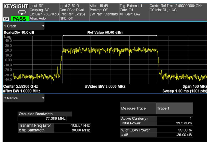
Channel: MIDDLE, Modulation: 64QAM, BW=80MHz
