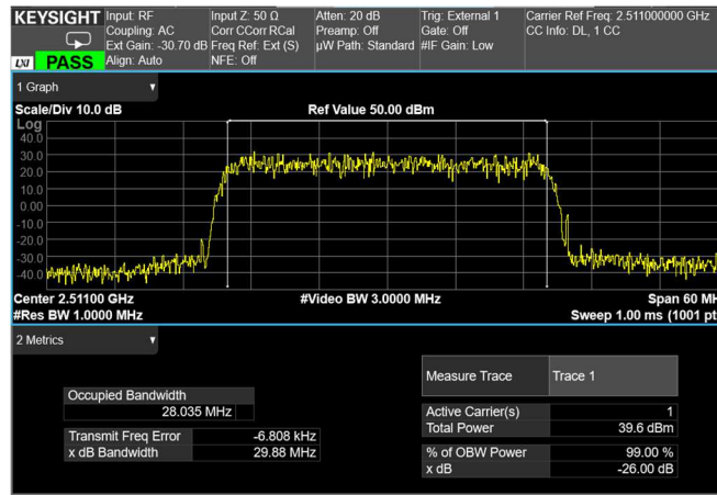
Channel: BOTTOM, Modulation: 64QAM, BW=30MHz
