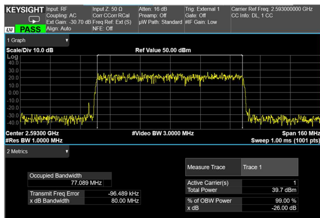
Channel: MIDDLE, Modulation: 64QAM, BW=80MHz
