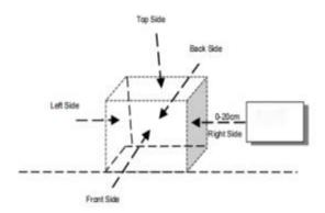
Note: Perform H-field measurements for each edge/top surface of the host/client pair at every 2 cm, starting from as close as possible out to 20 cm
