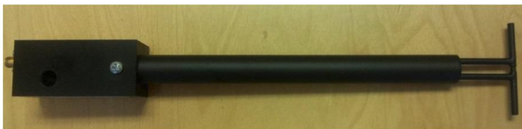
Figure 1 – MVG COMOSAR Validation Dipole
