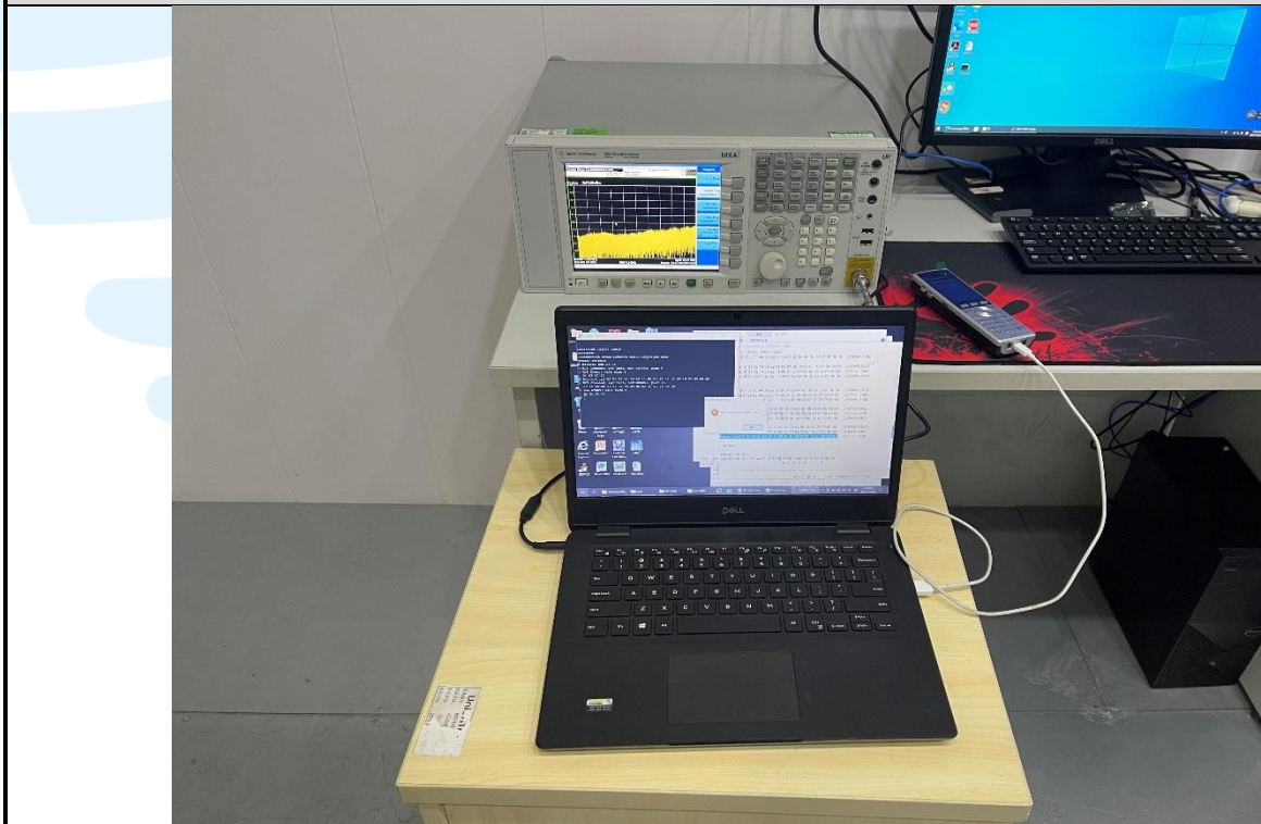
RF Conducted Test Setup
