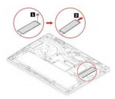
Type 2 Remove the screw and remove the M.2 solid-state drive bracket, and then remove the M.2 solid-state drive.
