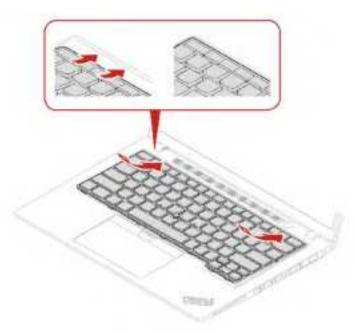
3. Slide the keyboard in the direction as shown. Ensure that the latches are secured under the keyboard frame.
