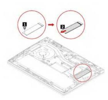
Type 2 Remove the screw and remove the M.2 solid-state drive bracket, and then remove the M.2 solid-state drive.
