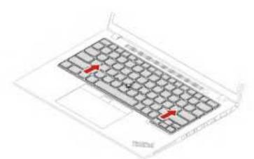
3. Pivot the keyboard slightly upward  $\blacksquare$  and then turn over the keyboard  $\blacksquare$ .
