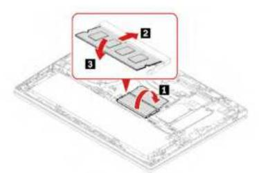
Note: For ThinkPad T14 Gen 5 Intel models, memory module replacement might cause memory retraining. For details, see "Detect memory retraining (for Intel models only)" on page 39.
