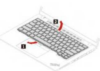
4. Put the keyboard on the palm rest as shown and detach the connectors. Then, remove the keyboard.
