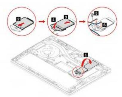
Note: When you install the wireless WAN card, ensure that you connect the blue cable to connector AUX and the orange cable to connector MAIN.
