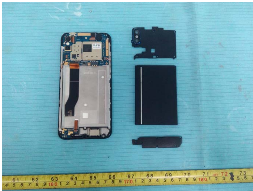
EUT – Cover off View 2
