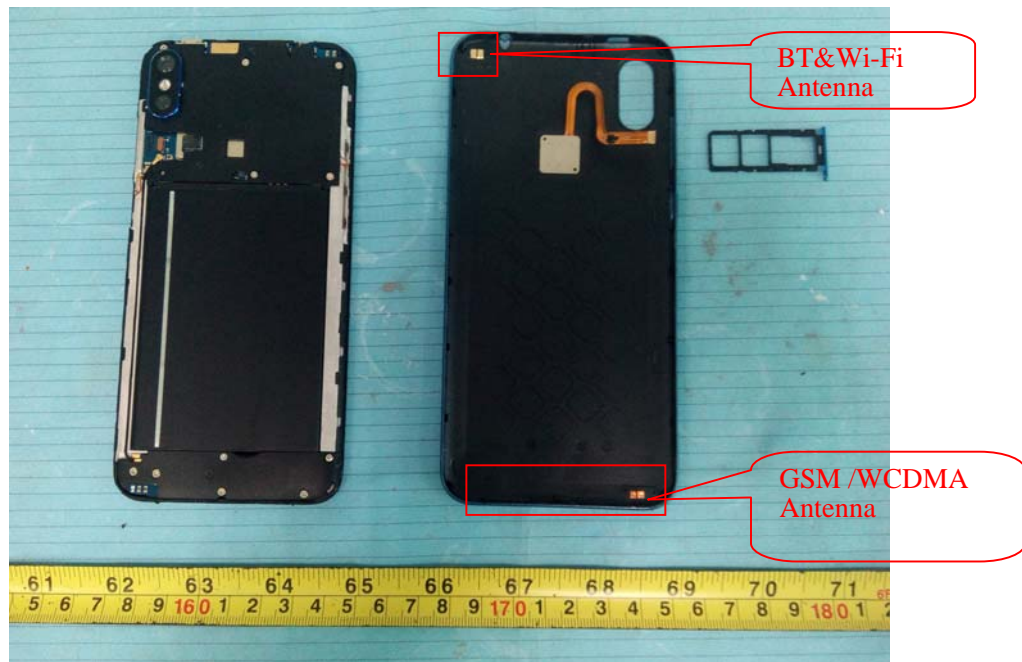
EUT – Cover off View 1
