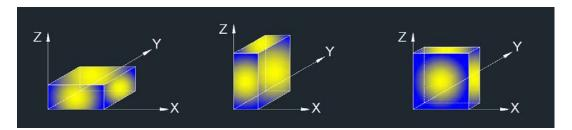
Note 1: For radiated test, EUT in each of three orthogonal axis emissions had been tested, but only the worst case (X axis) data recorded in the report.
