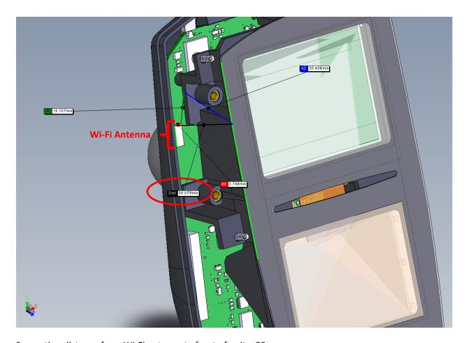
Separation distance from Wi-Fi antenna to front of unit = 39mm
