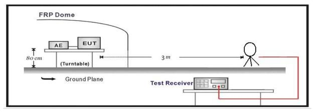
Below 1GHz Test Setup:
