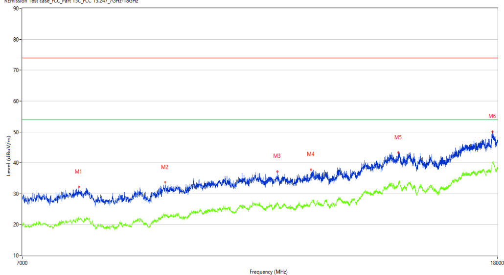
REmission Test case_FCC_Part 15C_FCC 15.247_7GHz-18GHz
