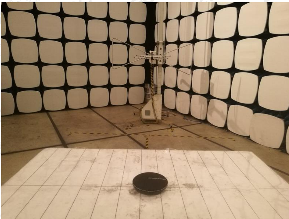
FCC RADIATED EMISSION TEST SETUP
