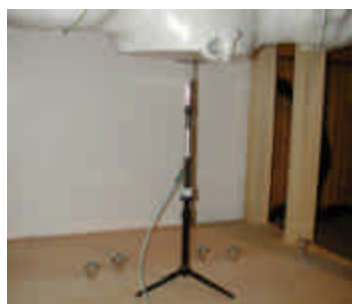
Figure 12.1 Dipole Validation Test Setup
