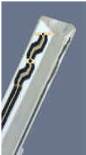
Figure 3.2 Probe Thick-Film Technique
