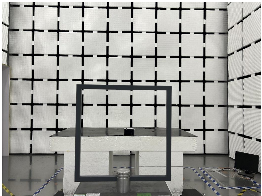
Radiation Emission Test Setup (Below 30MHz)
