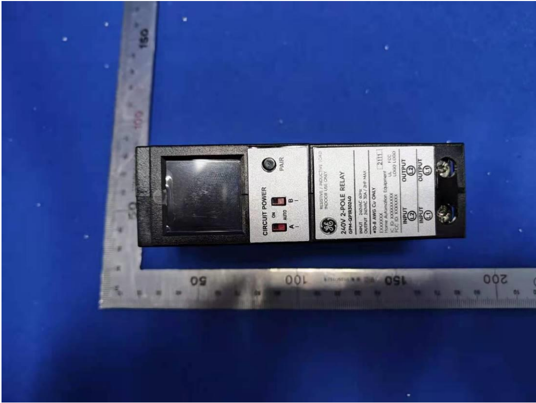
FIGURE 2 QO 240V 2-POLE RELAY, WITH CT, PON (M/N: GPM-QP1R30240-21) FRONT
