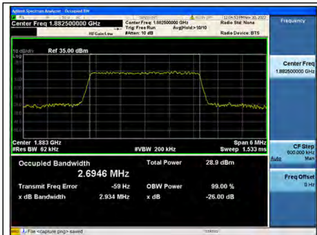
Band25 / 3MHz / QPSK/ Mid CH
