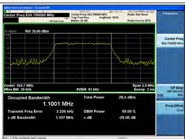
Band5 / 1.4MHz / 16QAM/ Low CH
