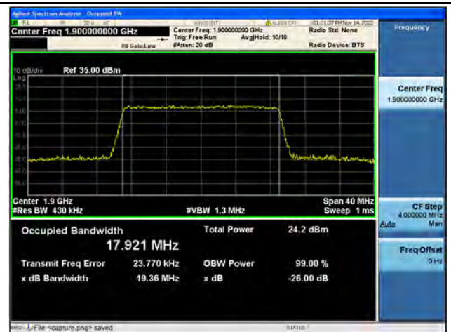
Band2 / 20MHz / 64QAM/ High CH
