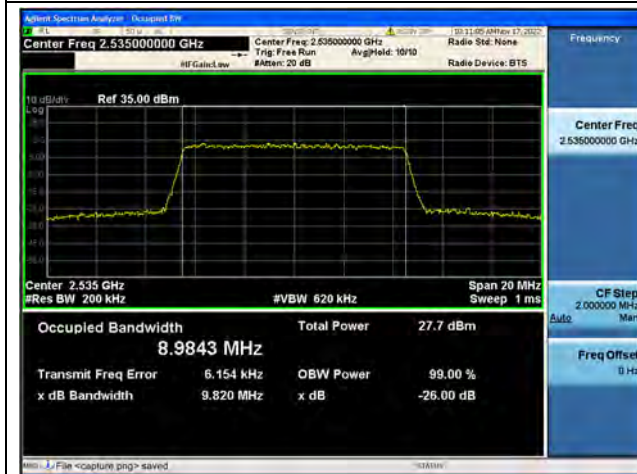
Band7 / 10MHz / 64QAM/ Mid CH
