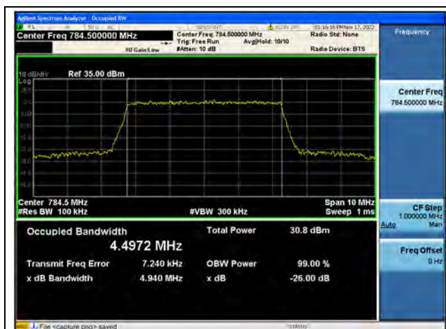
Band13 / 5MHz / QPSK/ High CH
