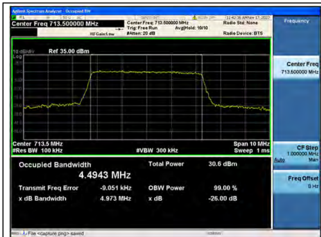
Band12 / 5MHz / QPSK/ High CH
