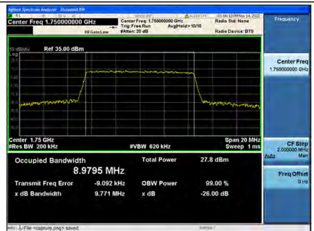
Band4 / 10MHz / 64QAM/ High CH
