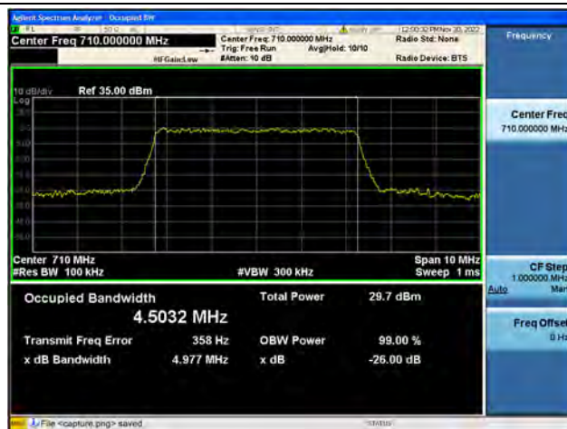
Band17 / 5MHz / 16QAM/ Mid CH
