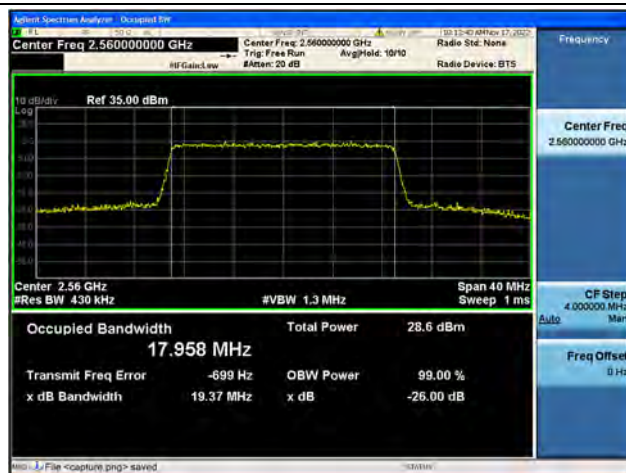
Band7 / 20MHz / 16QAM/ High CH
