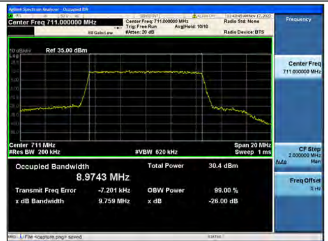
Band12 / 10MHz / QPSK/ High CH
