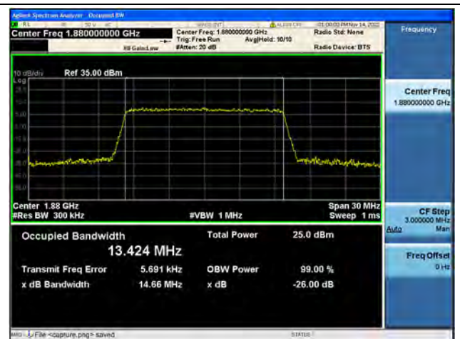
Band2 / 15MHz / 64QAM/ Mid CH
