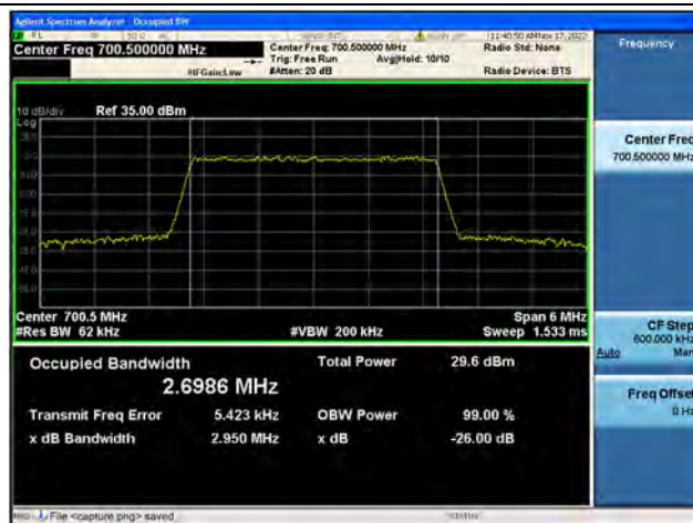
Band12 / 3MHz / 16QAM/ Low CH
