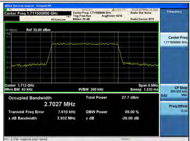
Band4 / 3MHz / 64QAM/ Low CH
