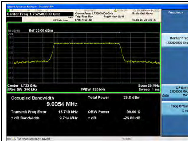
Band4 / 10MHz / QPSK/ Mid CH
