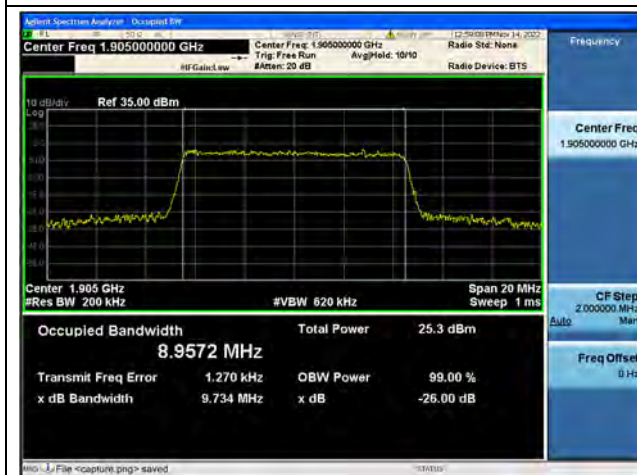
Band2 / 10MHz / 16QAM/ High CH
