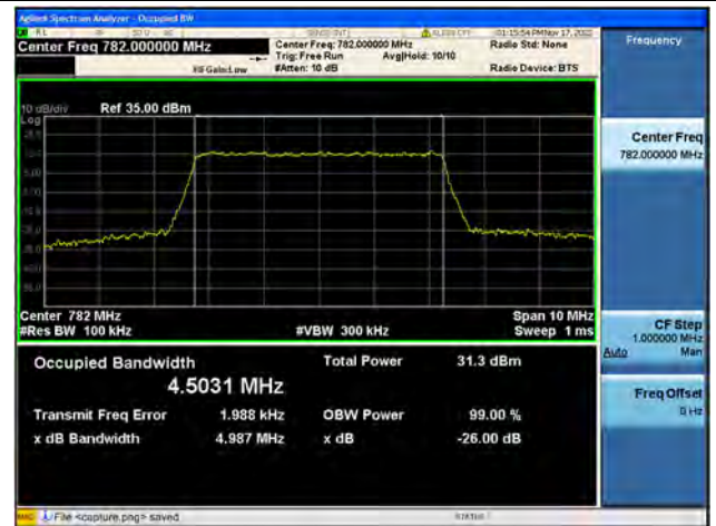
Band13 / 5MHz / QPSK/ Mid CH
