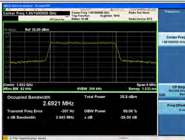
Band25 / 3MHz / 16QAM/ Low CH
