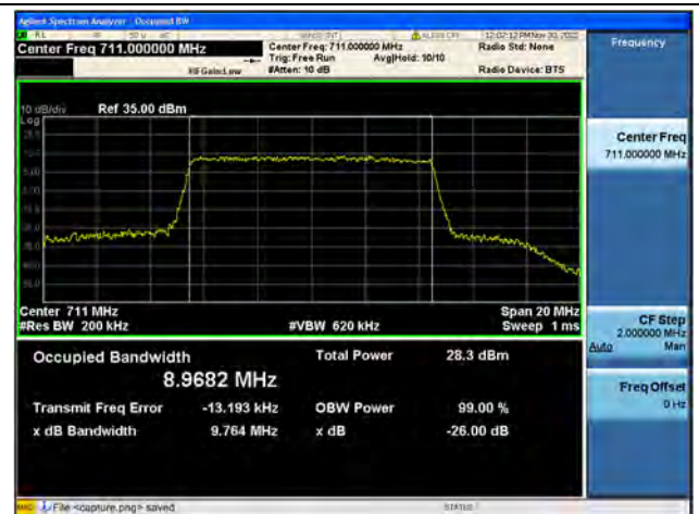
Band17 / 10MHz / 64QAM/ High CH
