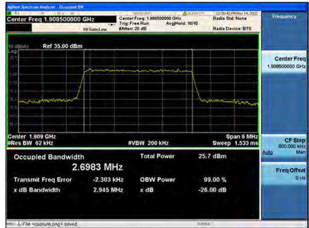
Band2 / 3MHz / QPSK/ High CH
