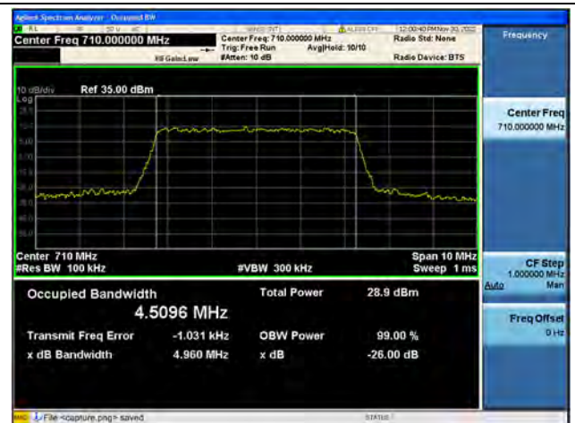
Band17 / 5MHz / 64QAM/ Mid CH
