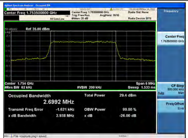
Band4 / 3MHz / QPSK/ High CH
