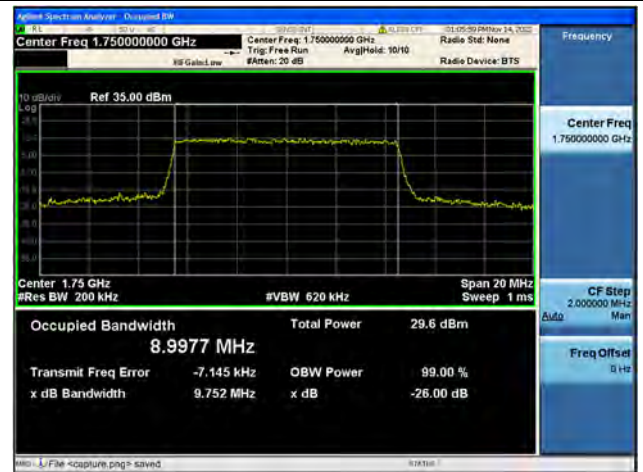
Band4 / 10MHz / QPSK/ High CH
