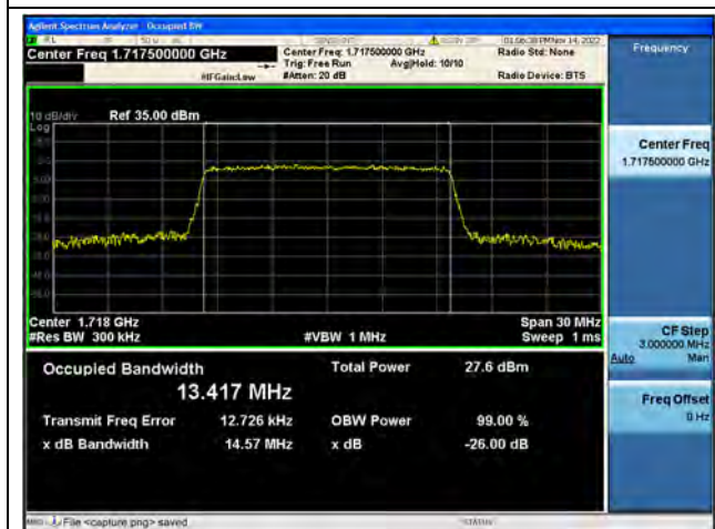
Band4 / 15MHz / 64QAM/ Low CH
