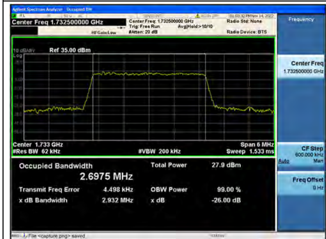
Band4 / 3MHz / 64QAM/ Mid CH
