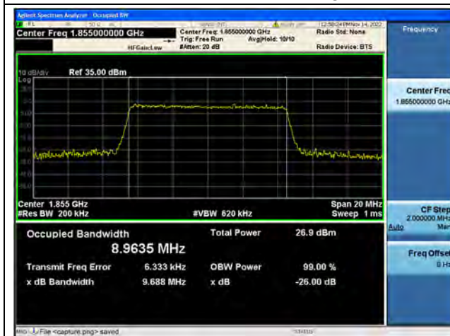
Band2 / 10MHz / 16QAM/ Low CH
