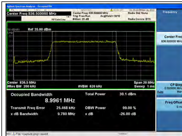
Band5 / 10MHz / QPSK/ Mid CH
