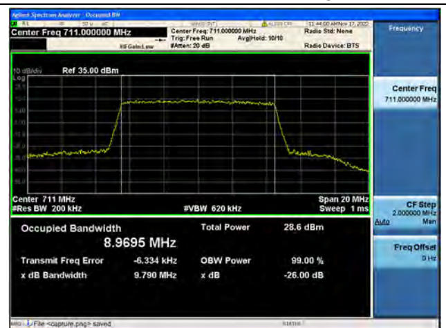
Band12 / 10MHz / 64QAM/ High CH
