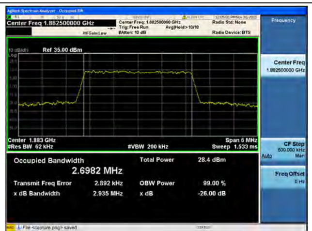
Band25 / 3MHz / 16QAM/ Mid CH
