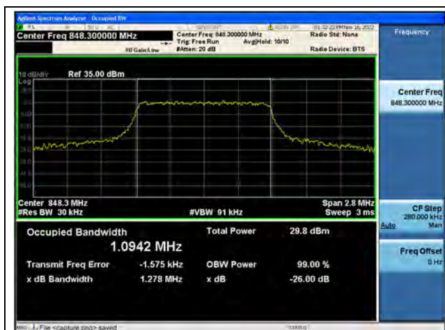
Band5 / 1.4MHz / QPSK/ High CH
