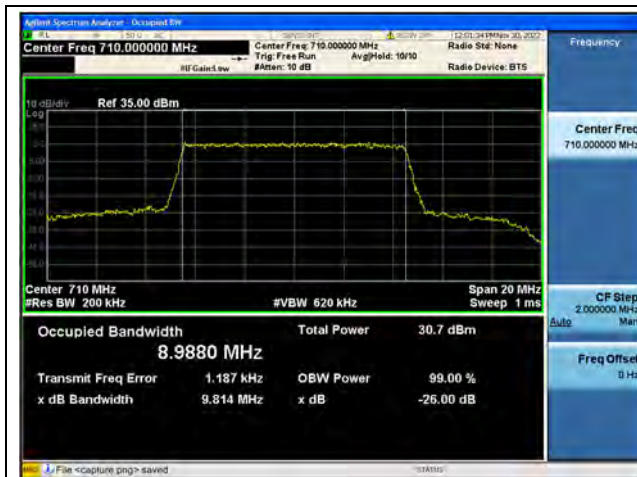
Band17 / 10MHz / QPSK/ Mid CH
