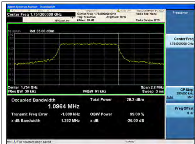
Band4 / 1.4MHz / QPSK/ High CH
