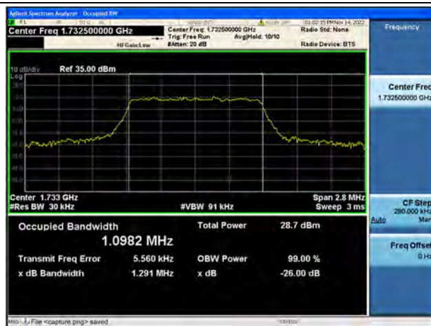
Band4 / 1.4MHz / 16QAM/ Mid CH
