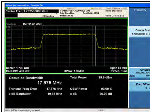
Band4 / 20MHz / QPSK/ Mid CH
