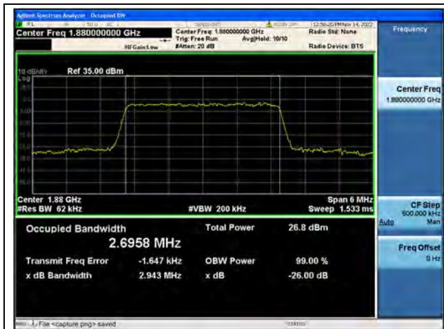
Band2 / 3MHz / QPSK/ Mid CH
