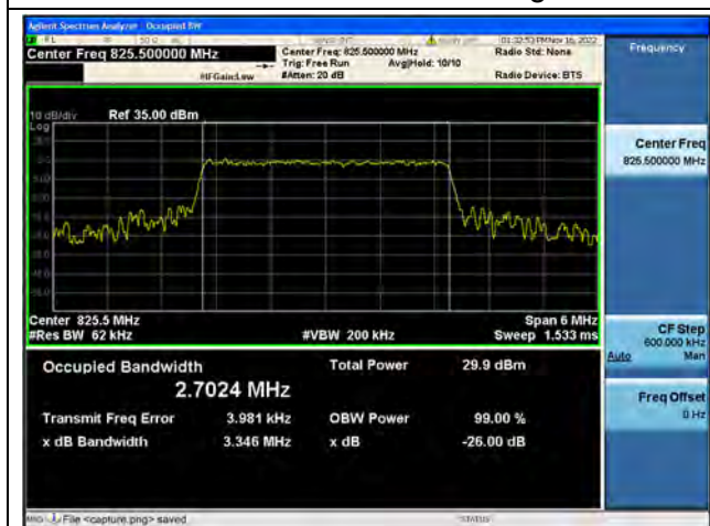
Band5 / 3MHz / 16QAM/ Low CH
