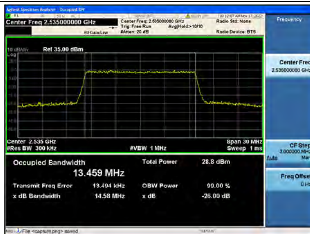
Band7 / 15MHz / 16QAM/ Mid CH
