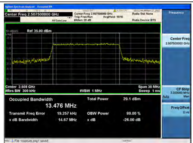
Band7 / 15MHz / 16QAM/ Low CH
