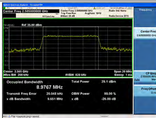
Band7 / 10MHz / 16QAM/ Low CH
