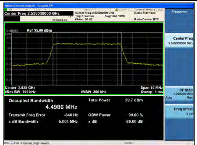
Band7 / 5MHz / QPSK/ Mid CH
