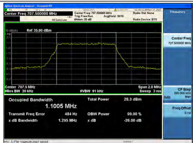
Band12 / 1.4MHz / 64QAM/ Mid CH
