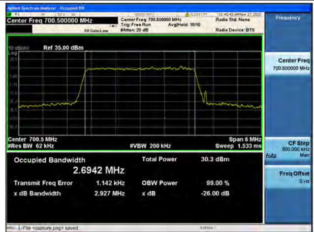
Band12 / 3MHz / QPSK/ Low CH
