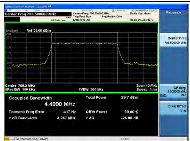
Band17 / 5MHz / 16QAM/ Low CH
