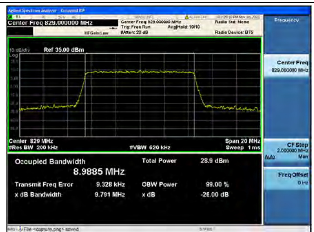
Band5 / 10MHz / 64QAM/ Low CH
