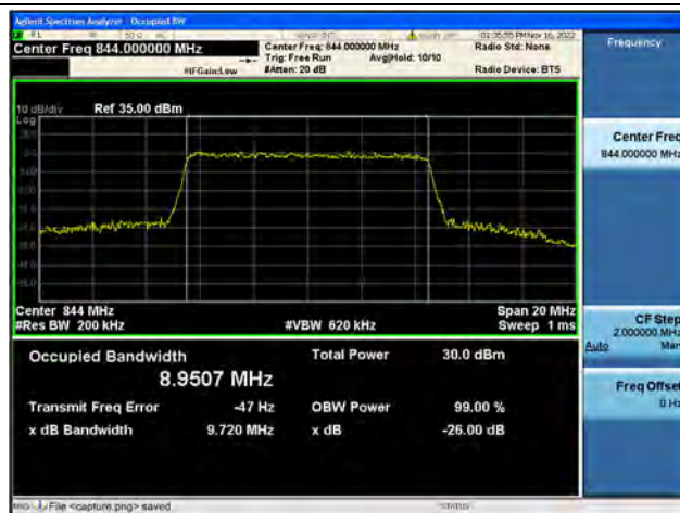
Band5 / 10MHz / 16QAM/ High CH
