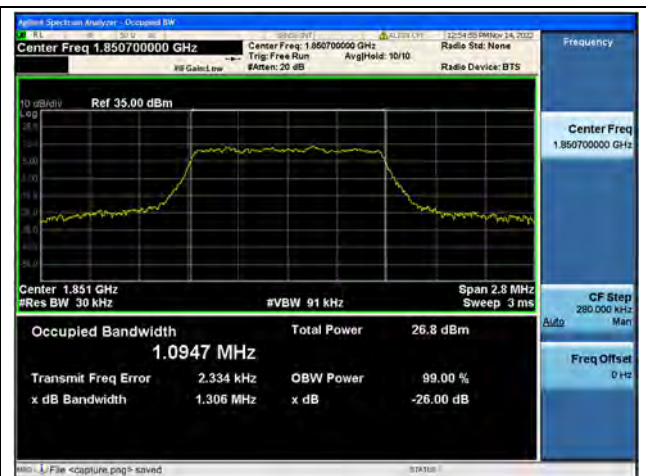
Band2 / 1.4MHz / 16QAM/ Low CH
