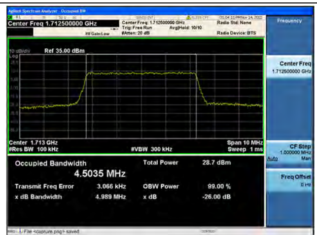
Band4 / 5MHz / 16QAM/ Low CH
