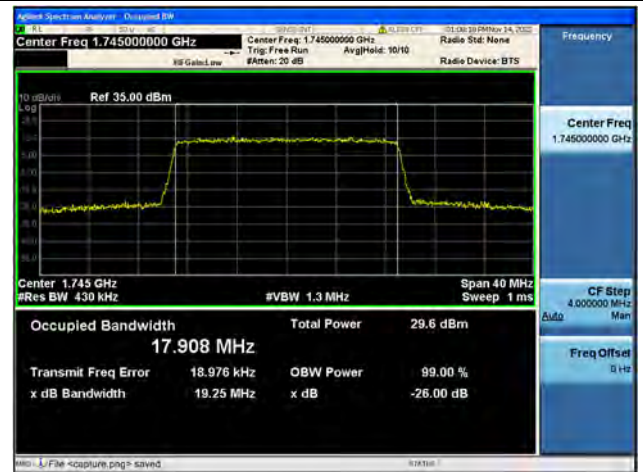
Band4 / 20MHz / QPSK/ High CH
