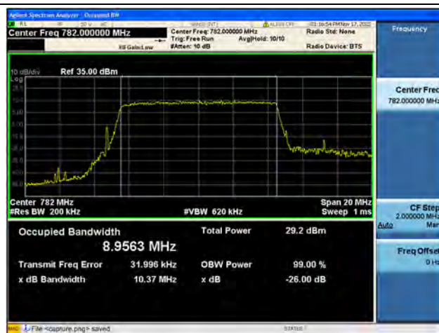
Band13 / 10MHz / 64QAM/ Low CH
