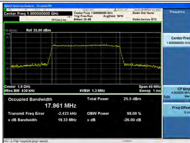
Band2 / 20MHz / 16QAM/ High CH
