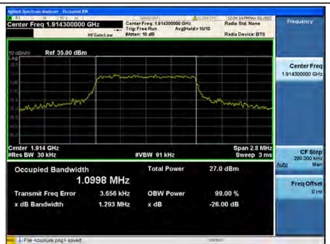
Band25 / 1.4MHz / 16QAM/ High CH
