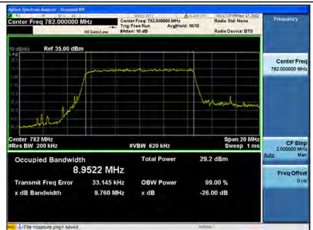
Band13 / 10MHz / 64QAM/ High CH
