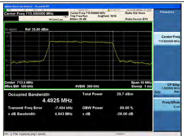
Band12 / 5MHz / 16QAM/ High CH
