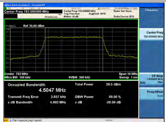
Band13 / 5MHz / 64QAM/ Mid CH
