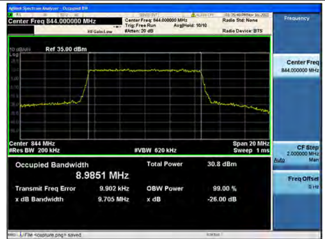
Band5 / 10MHz / QPSK/ High CH
