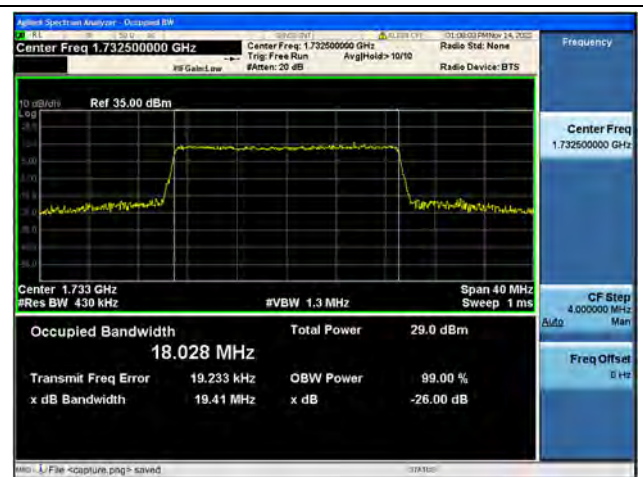
Band4 / 20MHz / 16QAM/ Mid CH
