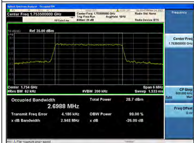
Band4 / 3MHz / 16QAM/ High CH
