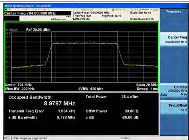
Band12 / 10MHz / 64QAM/ Low CH
