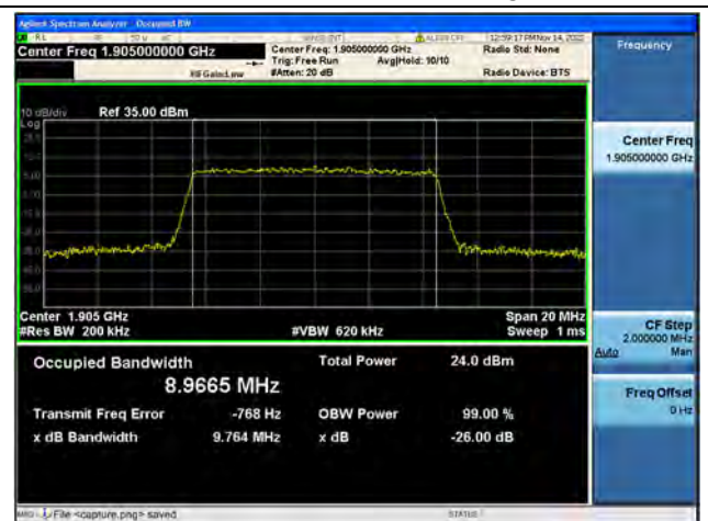
Band2 / 10MHz / 64QAM/ High CH
