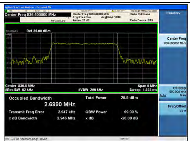
Band5 / 3MHz / 16QAM/ Mid CH
