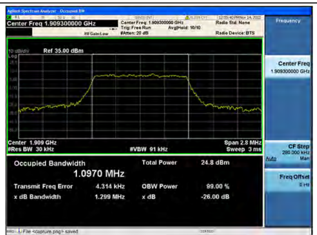
Band2 / 1.4MHz / 16QAM/ High CH
