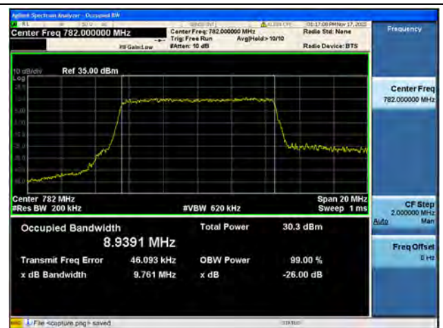
Band13 / 10MHz / 16QAM/ Mid CH
