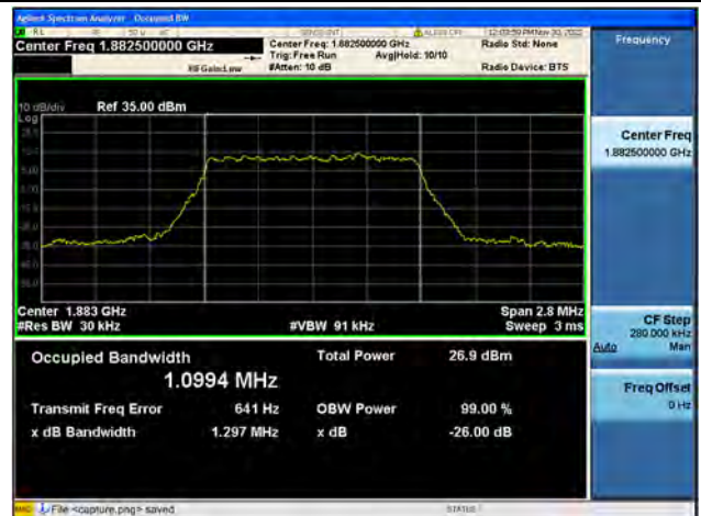
Band25 / 1.4MHz / 64QAM/ Mid CH
