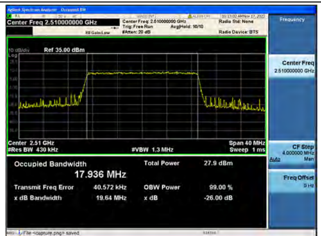
Band7 / 20MHz / 64QAM/ Low CH
