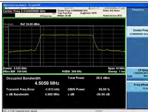
Band7 / 5MHz / 16QAM/ Mid CH
