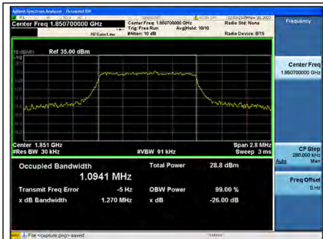
Band25 / 1.4MHz / QPSK/ Low CH
