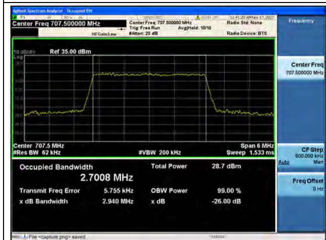
Band12 / 3MHz / 64QAM/ Mid CH
