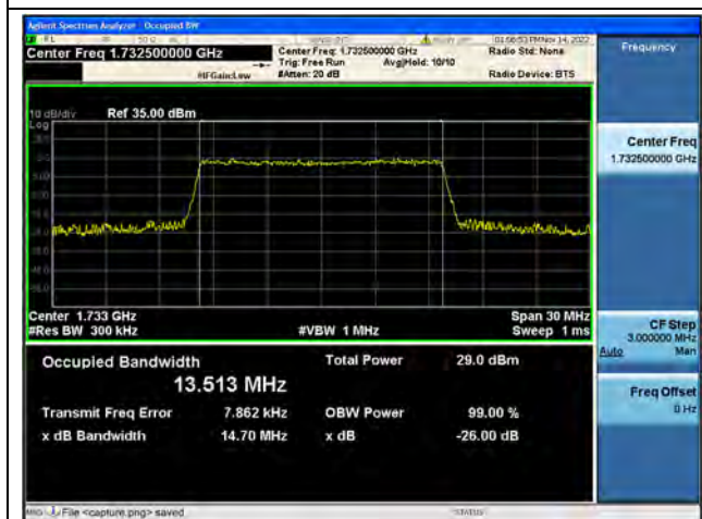
Band4 / 15MHz / 16QAM/ Mid CH
