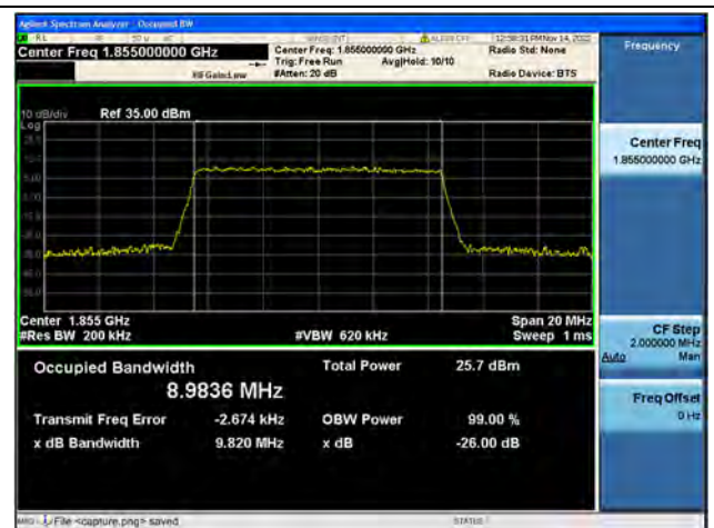
Band2 / 10MHz / 64QAM/ Low CH
