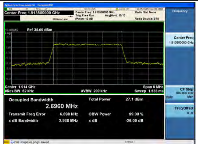
Band25 / 3MHz / 64QAM/ High CH
