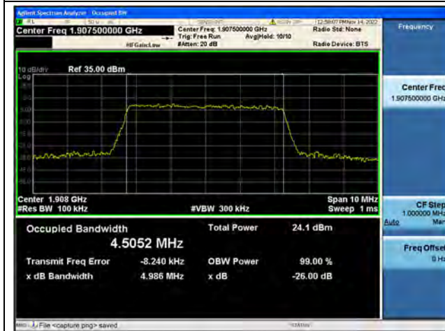
Band2 / 5MHz / 64QAM/ High CH
