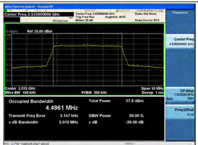
Band7 / 5MHz / 64QAM/ Mid CH
