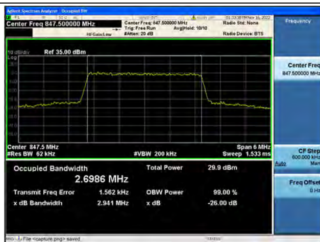
Band5 / 3MHz / 16QAM/ High CH
