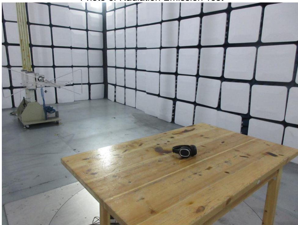
Photo of Radiation Emission Test
