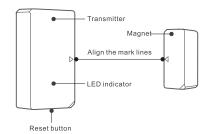
SNZB-04P is a Zigbee low-energy wireless door/window sensor that makes you know the opening/closing status of door and window by separating the magnet from the transmitter. Connect it with the Bridge and you can create a smart scene to trigger other devices.
