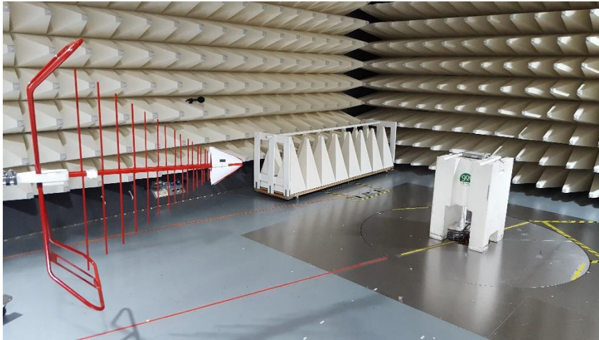
Figure B4. Low Range Radiated Emission test setup
