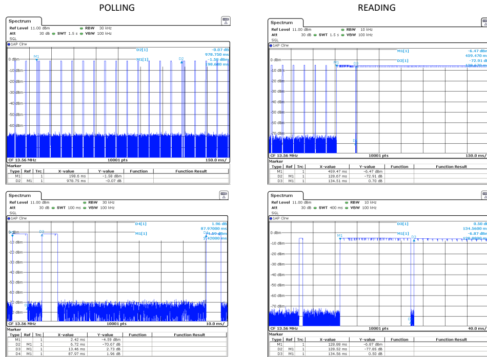
Figure 4.2.1 Example Pulsed Emission Characteristics (Duty Cycle).
