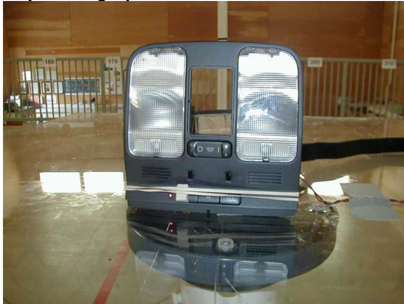
Figure 5.1 EUT in the "End" orientation.
