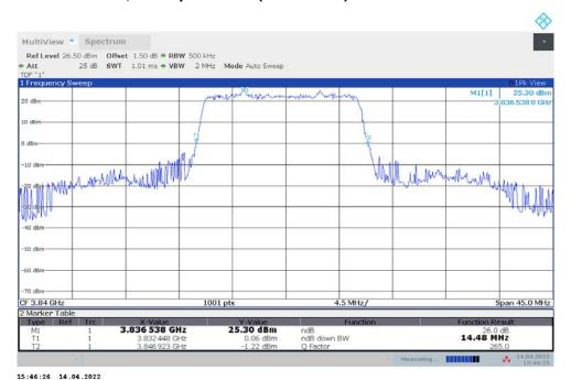
n77H,15MHz Bandwidth,DFT-s-QPSK (-26dBc BW)
