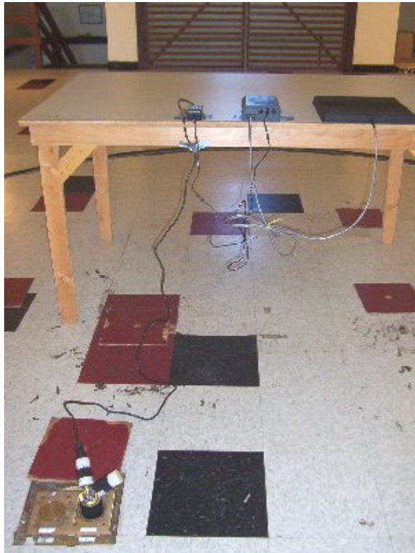
Radiated Emissions Test Setup – Rear View
