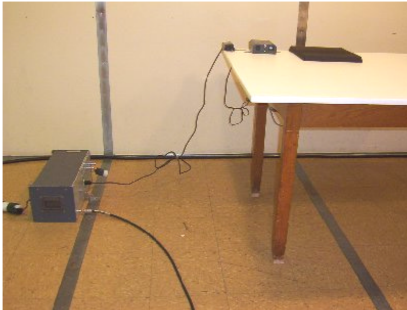
Conducted Emission Test Setup
