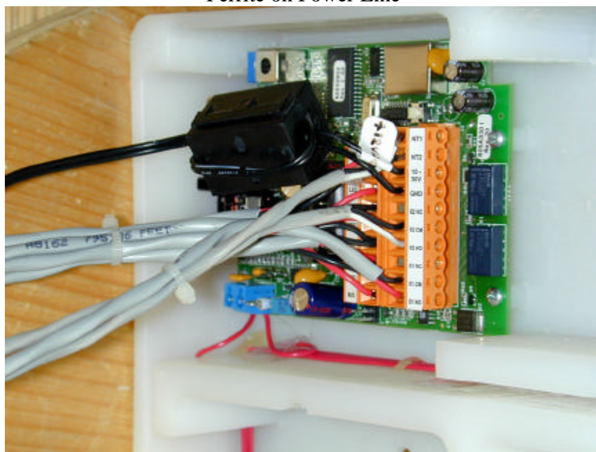
Ferrite on Power Line
