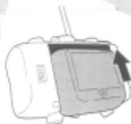
First, attach the CHARGER to the back of the CONTROLLER as shown.
