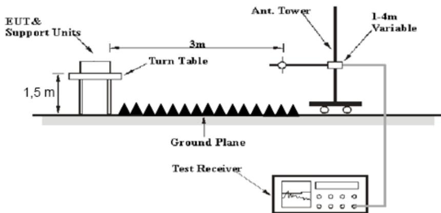
The radiated emission below 1GHz tests were performed in the 3 meters chamber test site A, above 1GHz tests were performed in the 3 meters chamber test site B, using the setup accordance with the ANSI C63.10-2013. The specification used was the FCC 15.209, and FCC 15.247 limits and the RSS-247 Clause 5.5, RSS-GEN Clause 8.10 limits.
