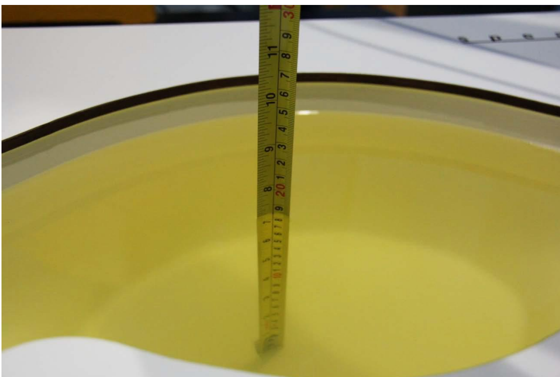
Picture 7-4: Liquid depth in the Flat Phantom(2450MHz)
