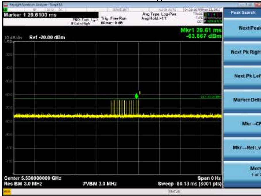
11ac80 CH106 5530MHz Radar Type 4 Calibration Plot
