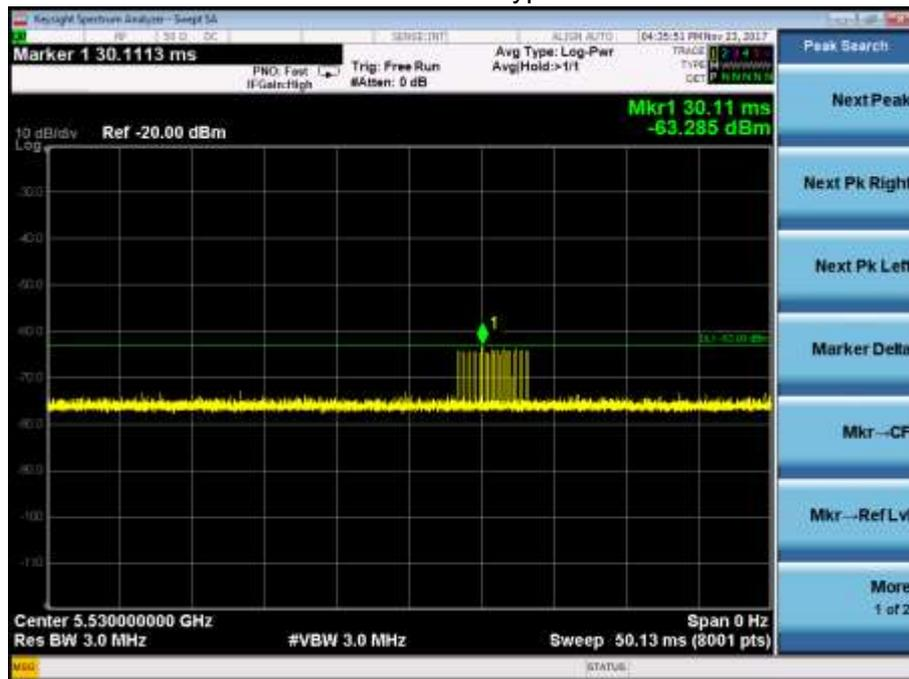
11ac80 CH106 5530MHz Radar Type 3 Calibration Plot
