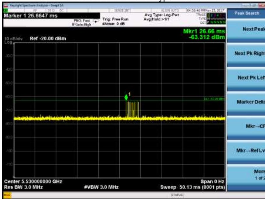
11ac80 CH106 5530MHz Radar Type 5 Calibration Plot
