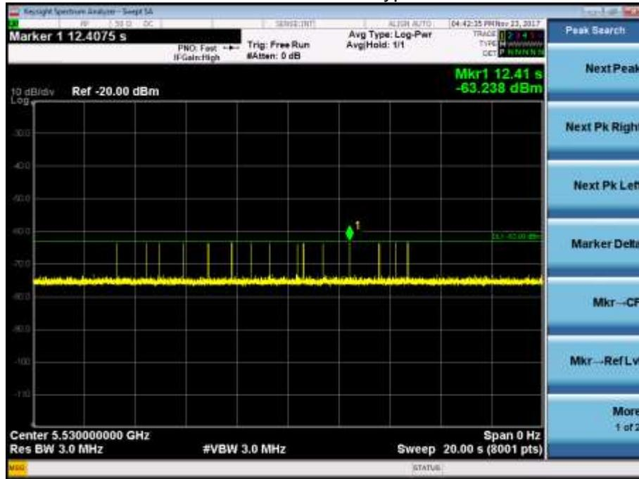
11ac80 CH106 5530MHz Radar Type 6 Calibration Plot
