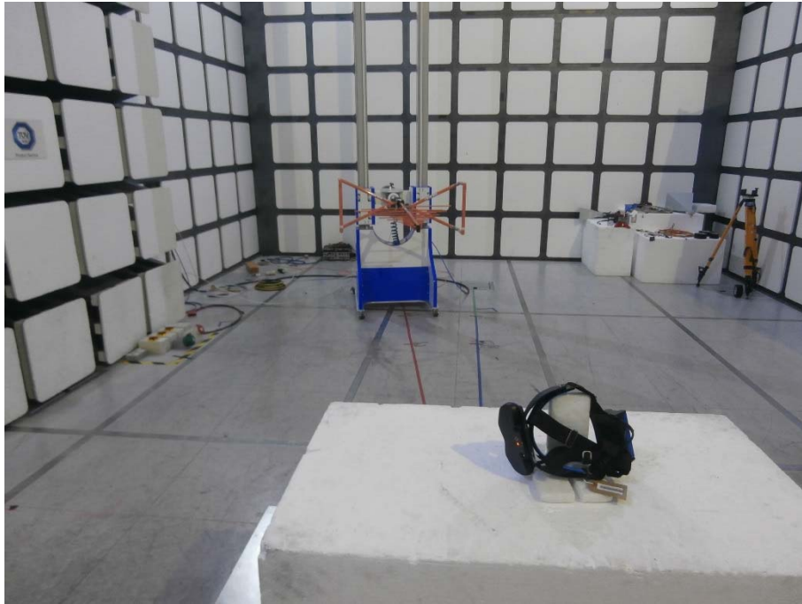
Radiated Emissions 30 MHz to 1 GHz
