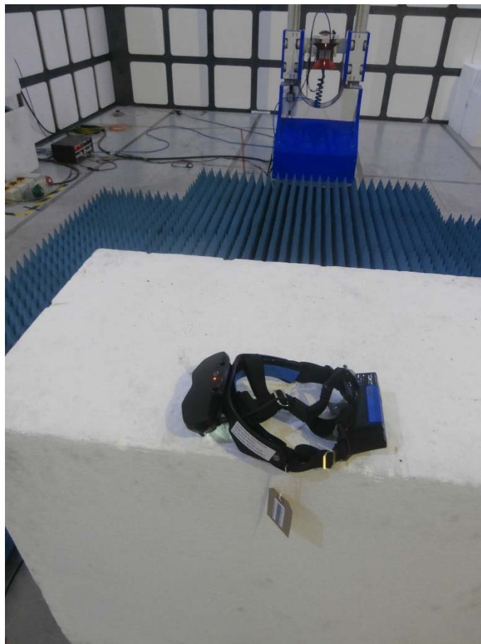
Radiated Emissions 1 GHz to 18 GHz
