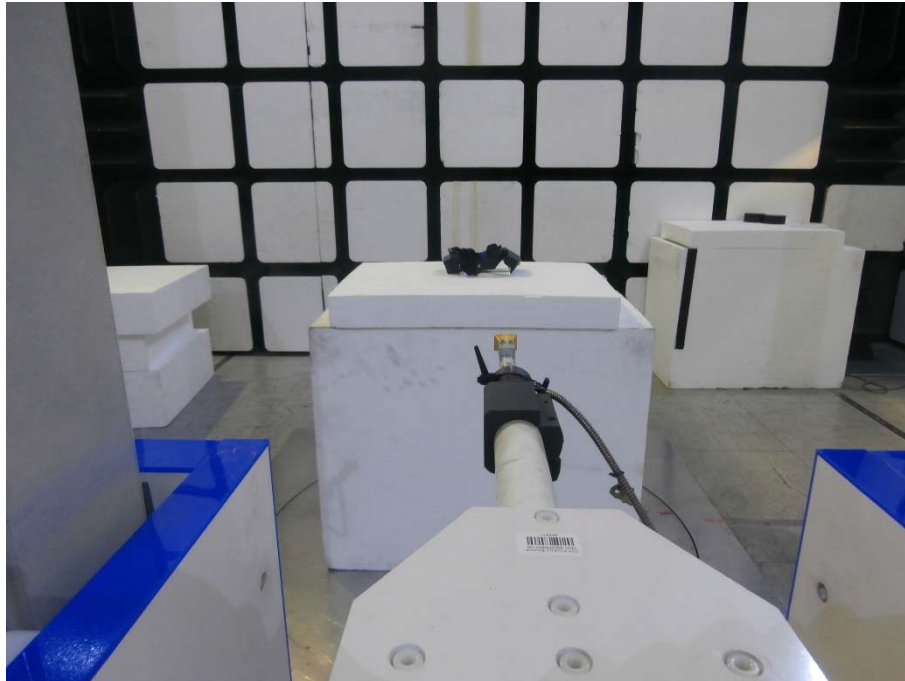
Radiated Emissions 18 GHz to 30 GHz
