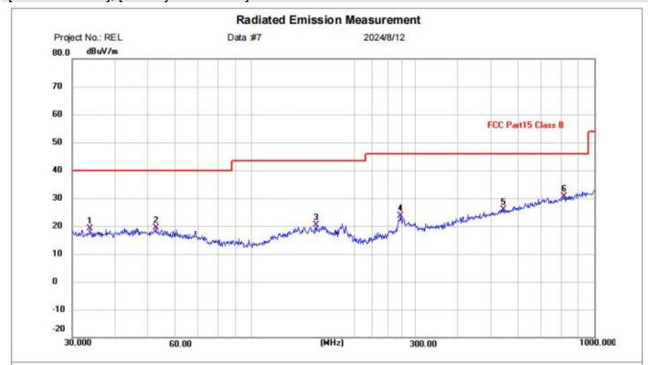
Site Polarization: Horizontal Temperature: (C)
