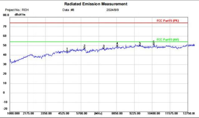
Site Polarization: Vertical Temperature: (C)
