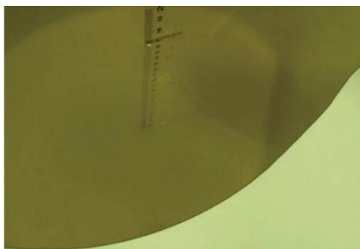
Picture 9.2-2: Liquid depth in the Flat Phantom ( Head 1750 MHz)
