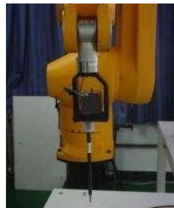
Picture 7-3 E-field Probe
