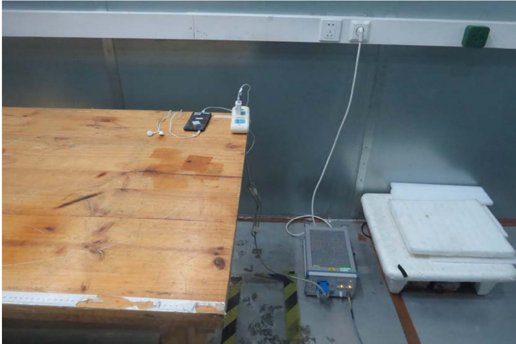
Picture 2 Conducted Emission Test Setup
