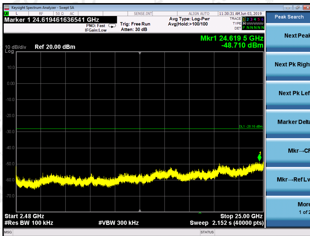
TEST PLOT OF OUT OF BAND EMISSIONS THE WORST CASE OF 802.11g FOR MODULATION IN HIGH CHANNEL
