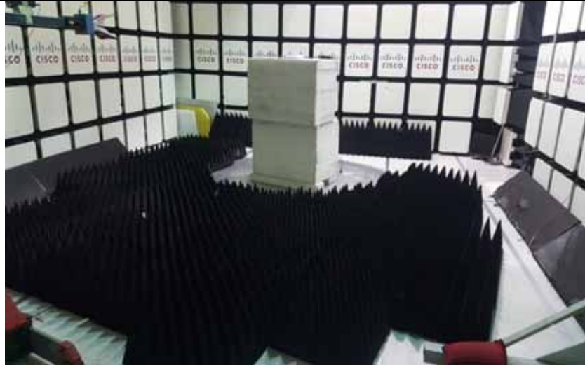
Radiated Setup 1GHz – 18GHz
