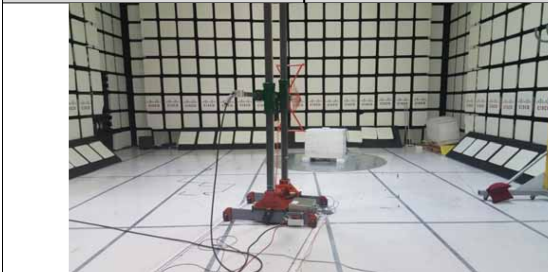
Radiated Setup 30MHz – 1GHz
