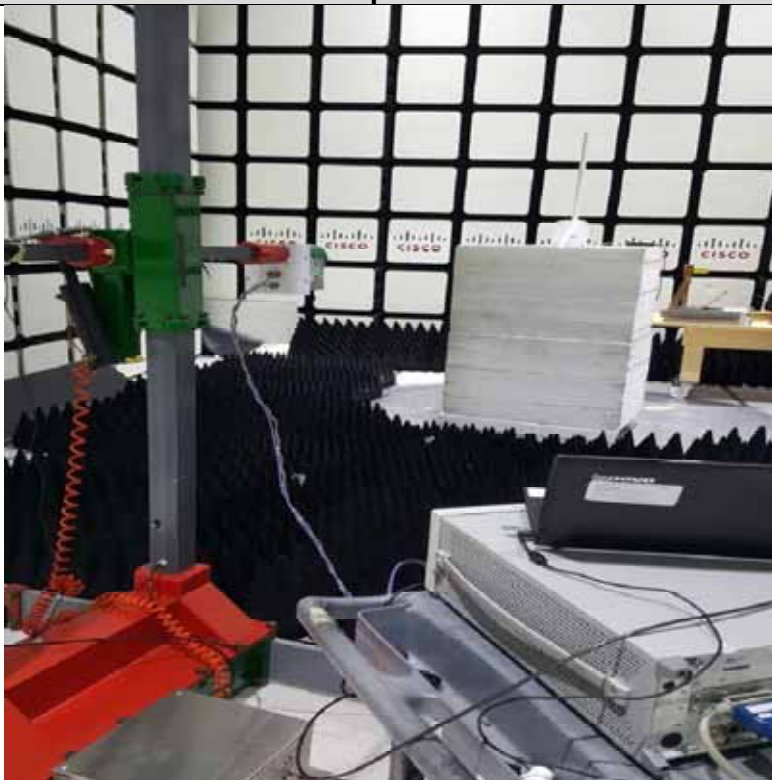
Radiated Setup 18GHz – 26GHz
