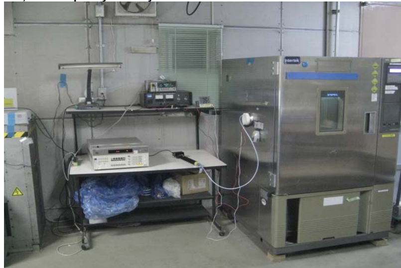
10.8, 10.9 Frequency Stability : Outer view
