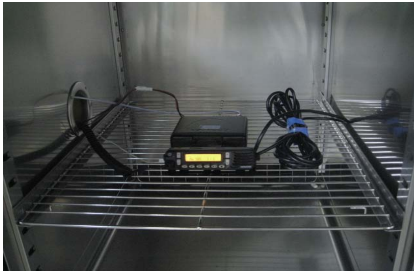
10.8, 10.9 Frequency Stability : Inner view
