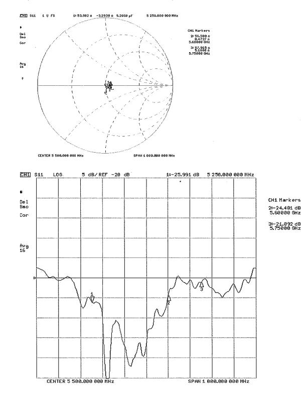
Impedance & Return-Loss Measurement Plot for Body TSL
