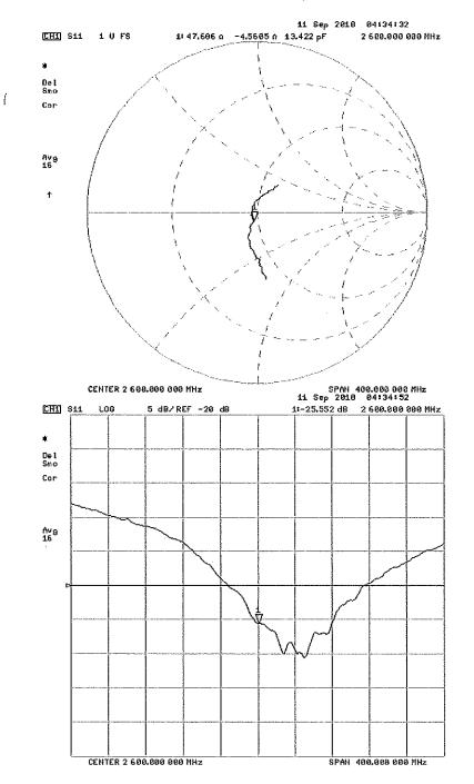
Impedance & Return-Loss Measurement Plot for Body TSL
