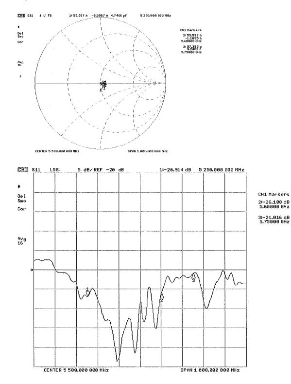
Impedance & Return-Loss Measurement Plot for Head TSL
