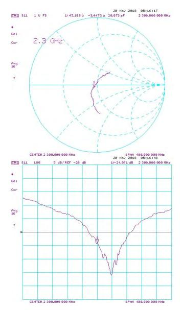
Impedance & Return-Loss Measurement Plot for Body TSL
