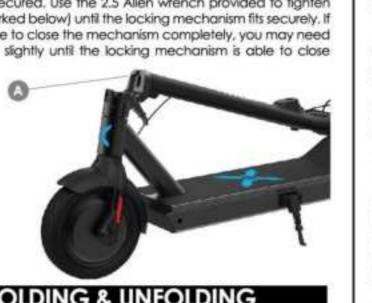
FOLDING & UNFOLDING To unfold your Renegade, press down on the folding clip and pull the steering column up. Raise the safety lock up and push it into place to secure the steering column. You will hear a "click", indicating the steering column is locked. Ensure the steering column is secured in
