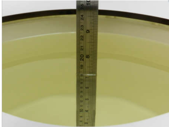
Fig 10.1 Photo of Liquid Height for Body SAR
